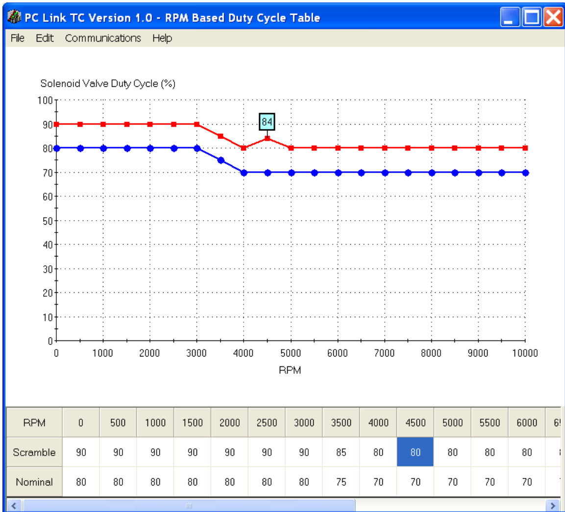
Figure 14 – RPM Based Duty Cycle Table
