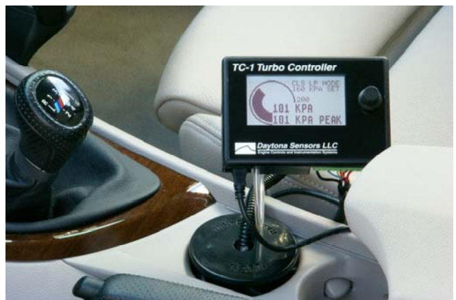
Figure 1 – Typical TC-1 Installation
