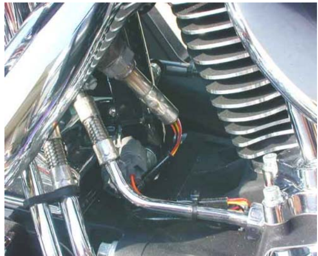
Figure 1 – Typical Sensor Installation
