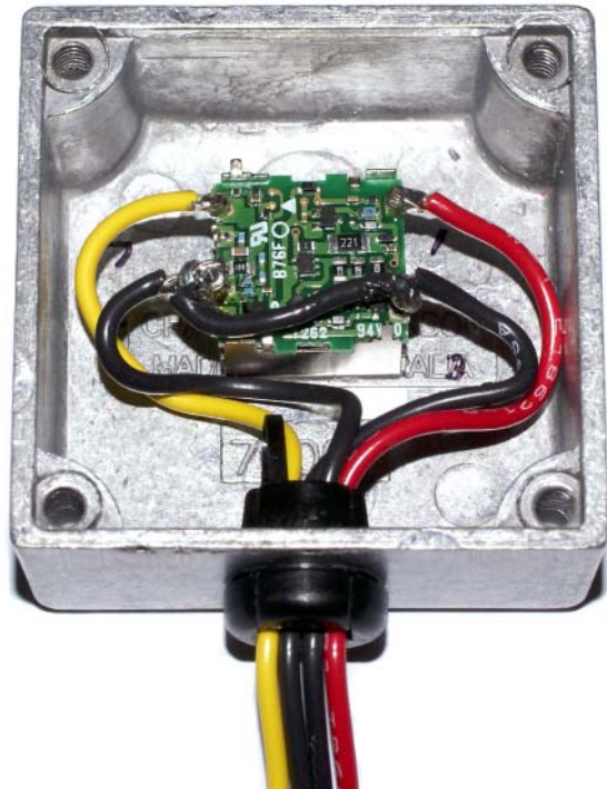
Figure 1 – Completed Auxiliary Power Supply
